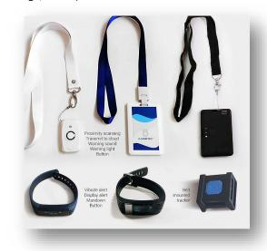
When a proximity is detected both devices will make a sound and vibrate, and they will send the other device's ID to a central server (that can be on premise or in the cloud). The data is not shared public and the solution is to be seen as a private network.
